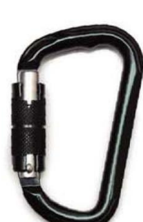
D1 Carabiner C3102 series Forged Aluminum Alloy Twist Lock Snag-free Design Anodized Min. Breaking Strength: 23kN/5000lbs
