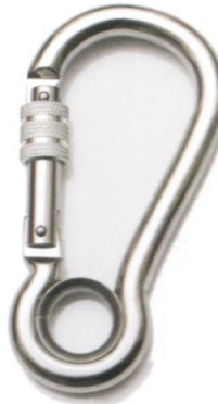
WAIST Carabiner C4201 series Alloy Steel Screw Lock Min. Breaking Strength: 23kN/5000lbs
