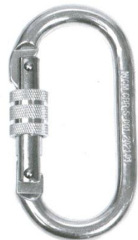
C Carabiner CBR-S-001 Alloy Steel Screw Lock Min. Breaking Strength: 23kN/5000lbs EN362 Certificated
