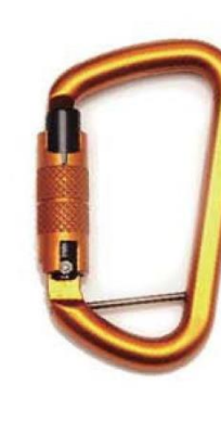
Carabiner C2102 series Aluminum Alloy With/Without Captive Pin Twist Lock Snag-free Design Anodized Min. Breaking Strength: 9kN/2000lbs
