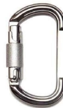
D Carabiner C2102 series Forged Aluminum Alloy Twist Lock Snag-free Design Anodized Min. Breaking Strength: 23kN/5000lbs
