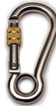
WAIST Carabiner C4301 series Stainless Steel(SUS 304) Screw Lock Min. Breaking Strength: 10kN/2500lbs
