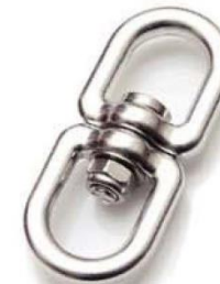
Aluminum Swivel Connector I0102 series Forged Aluminum Alloy Anodized Min. Breaking Strength: 9kN/2000lbs
