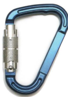
D1 Carabiner CBRAD1-ALF-001 Forged Aluminum Alloy Twist Lock Snag-Free Design Anodized Min. Breaking Strength: 23kN/5000lbs EN362 Certificated
