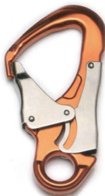
Self Locking Snap Hook RBH-M-AL-003 Forged Aluminum Alloy Anodized Min. Breaking Strength: 35kN/7500lbs EN362 Certificated
