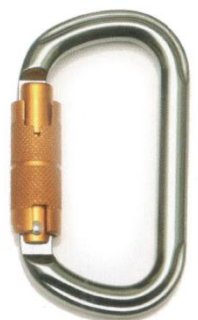
D Carabiner CBRAD-ALF-002 Forged Aluminum Alloy Twist Lock Snag-free Design Anodized Min. Breaking Strength: 23kN/5000lbs EN362 Certificated
