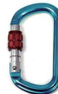
D Carabiner C2101 series Forged Aluminum Alloy Screw Lock Snag-free Design Anodized Min. Breaking Strength: 23kN/5000lbs
