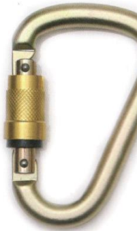
D1 Carabiner C3203 series Alloy Steel One-way Lock Min. Breaking Strength: 23kN/5000lbs
