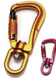
Swivel Connector I0201 series Forged Aluminum Alloy Twist Lock Snag-free Design Anodized Min. Breaking Strength: 9kN/2000lbs
