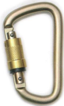
D Carabiner C2203 series Alloy Steel One-way Lock Min. Breaking Strength: 23kN/5000lbs
