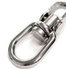
Swivel Combination I0202 series Alloy Steel Chrome Plated Min. Breaking Strength: 23kN/5000lbs
