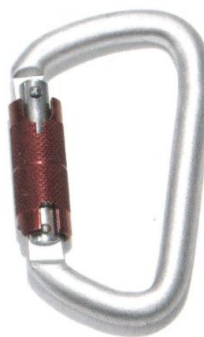
D1 Carabiner C3202 series Alloy Steel Twist Lock Min. Breaking Strength: 23kN/5000lbs
