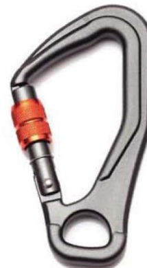
Screw Locking Snap Hook C5101 series Forged Aluminum Alloy Screw Lock Snag-free Design Anodized Titanium Min. Breaking Strength: 23kN/5000lbs
