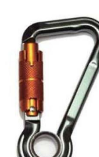
WAIST Carabiner C4102 series Forged Aluminum Alloy Twist Lock Snag-free Design Anodized Min. Breaking Strength: 23kN/5000lbs
