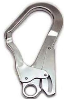
Self Locking Rebar Hook A0102 series Forged Alloy Steel Min. Breaking Strength: 23kN/5000lbs
