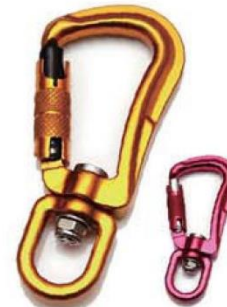
Swivel Connector I0201 series Forged Aluminum Alloy Twist Lock Snag-free Design Anodized Min. Breaking Strength: 9kN/2000lbs
