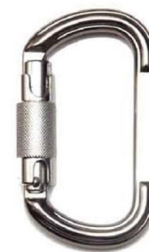
D Carabiner C2102 series Forged Aluminum Alloy Twist Lock Snag-free Design Anodized Min. Breaking Strength: 23kN/5000lbs
