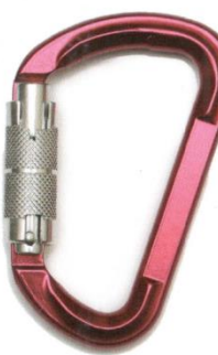
D1 Carabiner CBRAD1-ALF-004 Forged Aluminum Alloy Twist Lock Snag-free Design Anodized Min. Breaking Strength: 23kN/5000lbs EN362 Certificated
